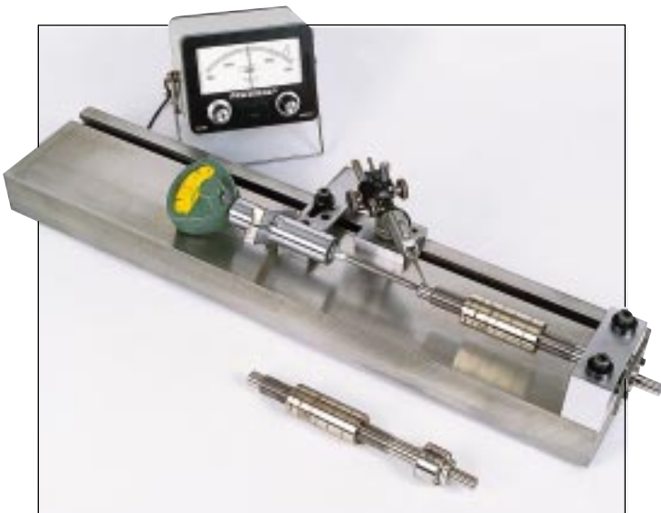
Inspection of bearing for thrust plane error.
